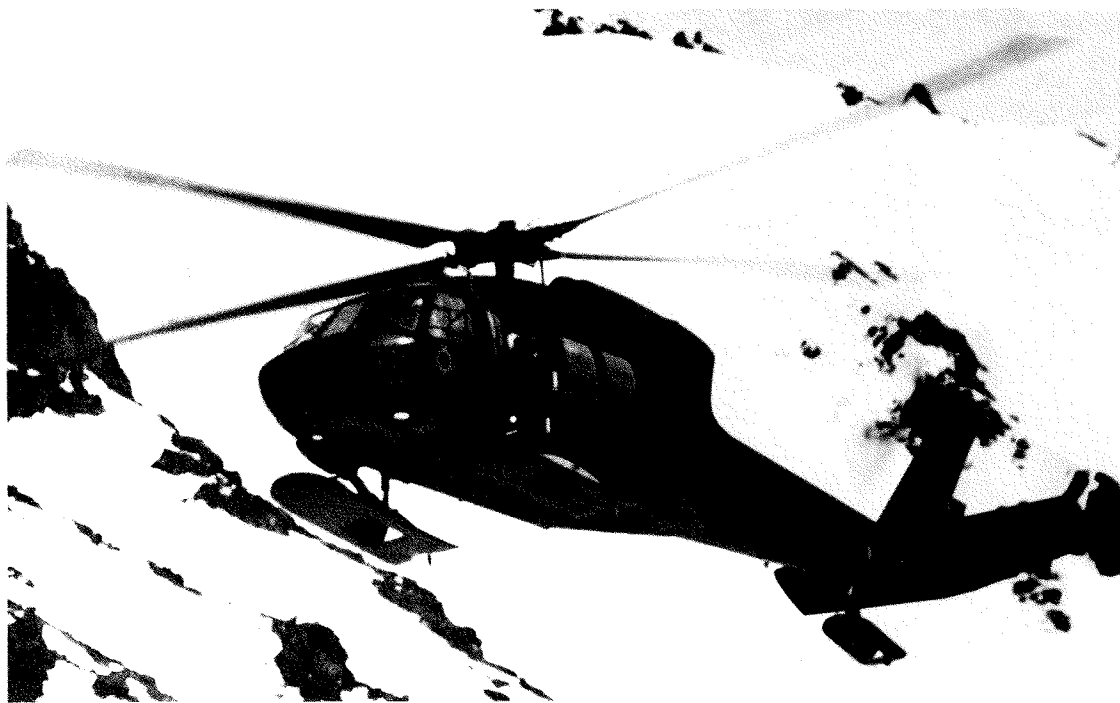
Skis have been adapted for the UH-60 Blackhawk helicopter for use in snow and on tundra.
