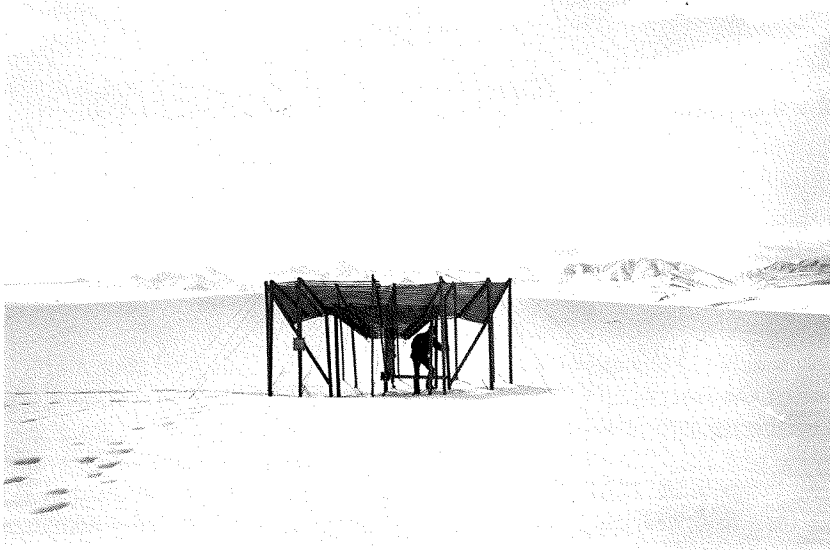
Wind-shielded snow gauge, Toolik River, northern Alaska.
