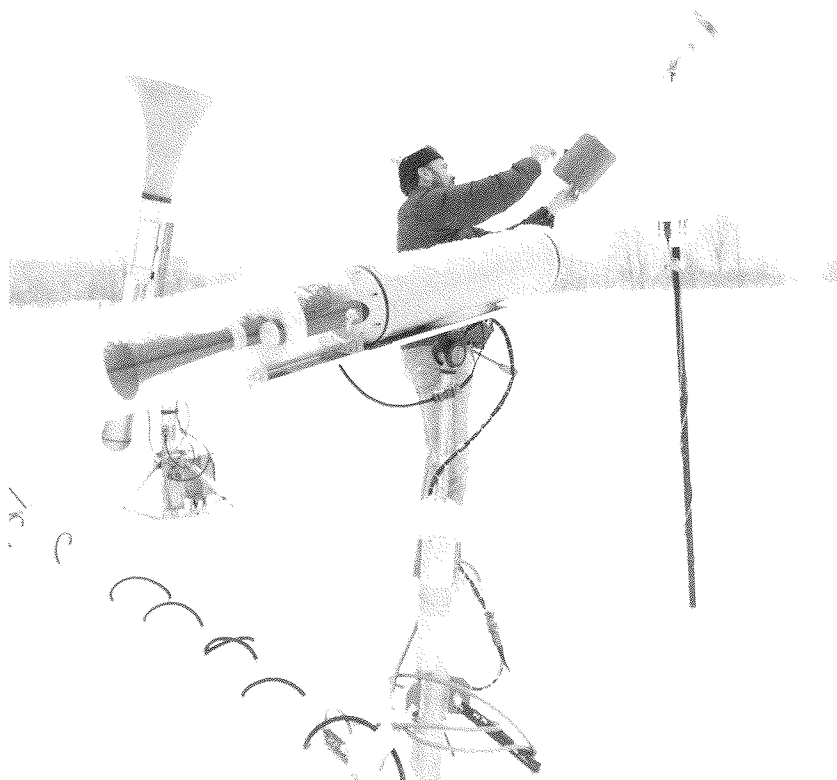
Instrumentation (Knollenberg probes) for determining snow crystal size, shape and concentration.
